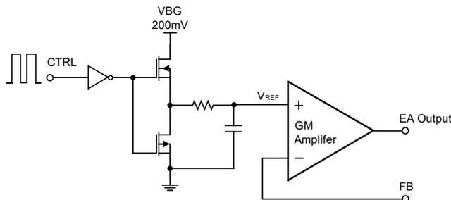
Figure 3. Programmable FB Voltage Using PWM Signal
