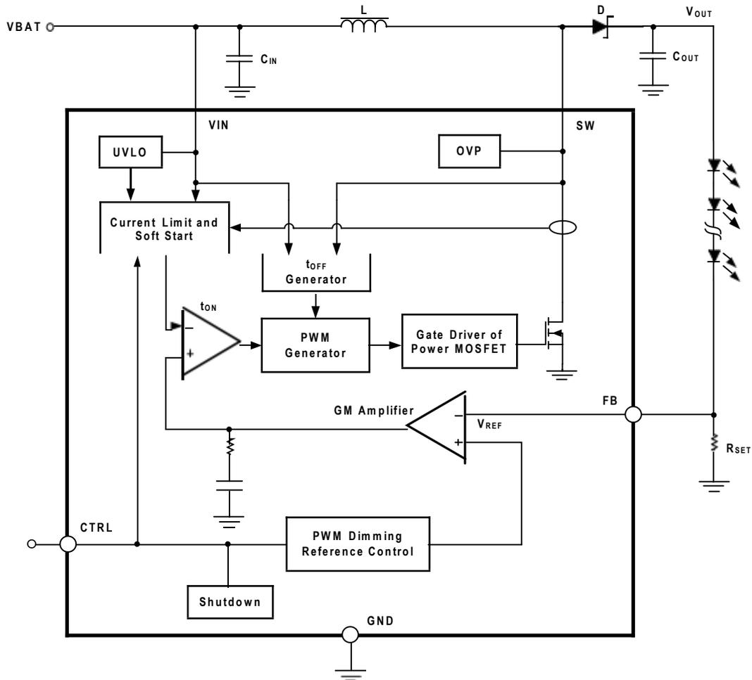
Figure 2. Block Diagram
